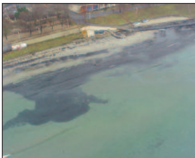
When oil becomes mixed with sediment, the density can become sufficiently high for it to sink if it is washed off the beach. In this photo, large patches of sunken oil are visible in shallow water close to the beach.
