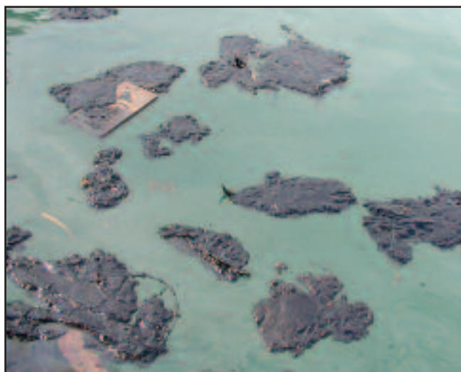
Oils spilled into the sea at temperatures below their pour point form solid fragments. This photo shows Nile Blend crude, pour point +33° C, in sea water of 28° C. Such oils are highly persistent and have the potential to travel great distances.
